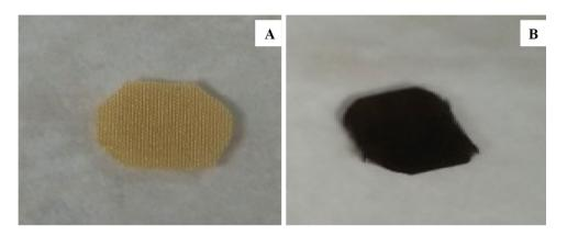
Fig. 3 Transformation of colour on the surface of textile fabric, with **a** 100% nylon before binded AgNPs and **b** 100% nylon after binded AgNPs
