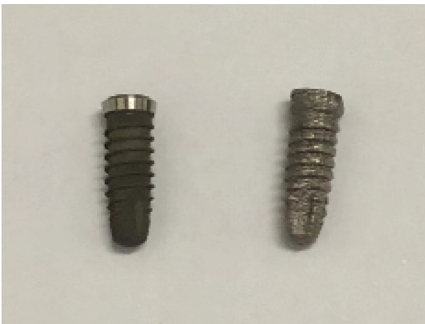
Fig. 2 The implant on the right in the picture is 3D printing of tantalum–niobium alloy dental implant primitive form; The dental implant on the left is the commonly used Ti alloy in clinic
