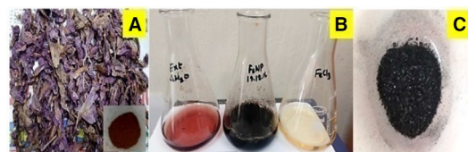
Fig. 1 Magnetite nanoparticle synthesis. a Dried hibiscus petals, inset: petal powder, b petal extract, nanoparticle solution as black precipitate and metal precursor solution, c calcined magnetite nanoparticles
