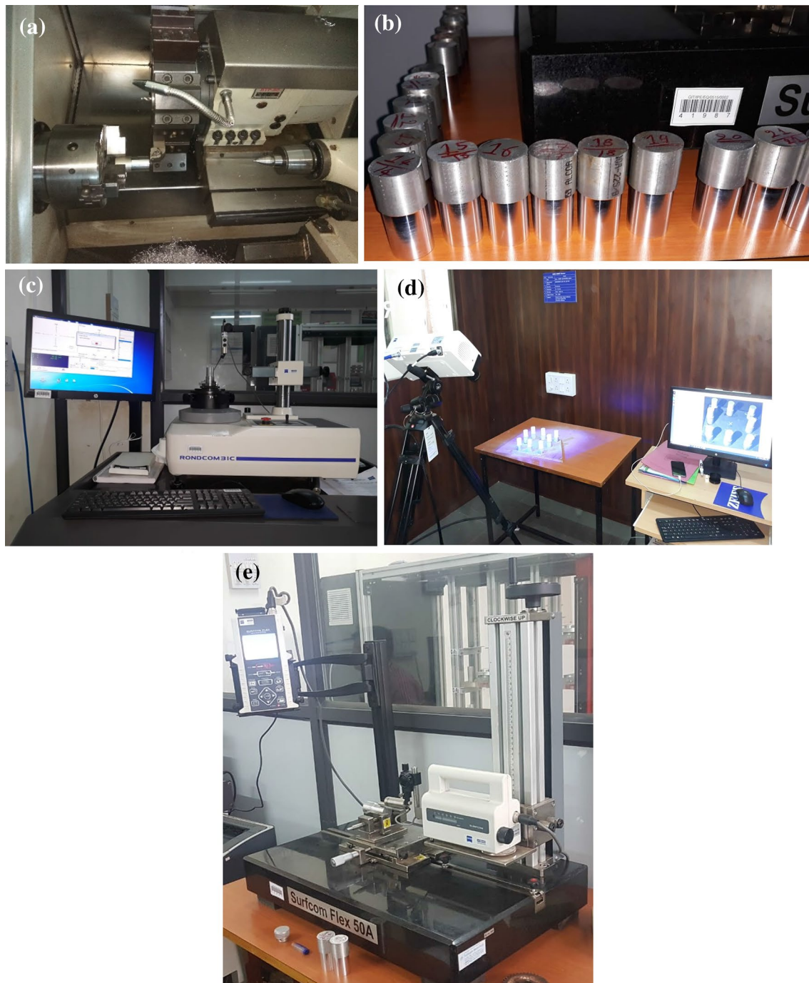
Fig. 1 a Experimental set-up, b turned parts, c circularity measurement device (ROND COM 31C), d cylindricity measurement device (COMET L3D Tripod a column type 3D Scanner) and e surface roughness test device (SurfCom Flex 50)
