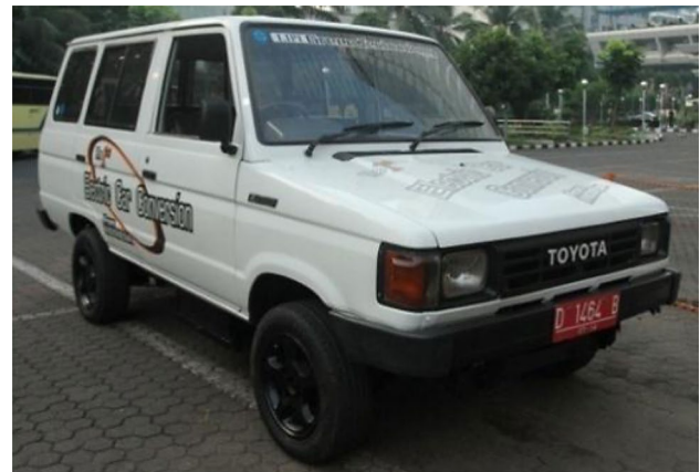
Fig. 1 1994 Toyota Kijang Super gasoline-to-electric converted car [26]
