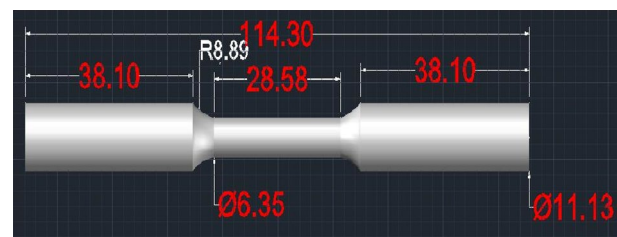
Fig. 1 Dimension of tensile sample
