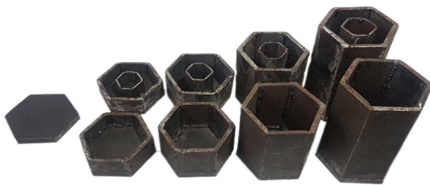
Fig. 4 Hexagonal footings unskirted, singly skirted and doubly skirted
