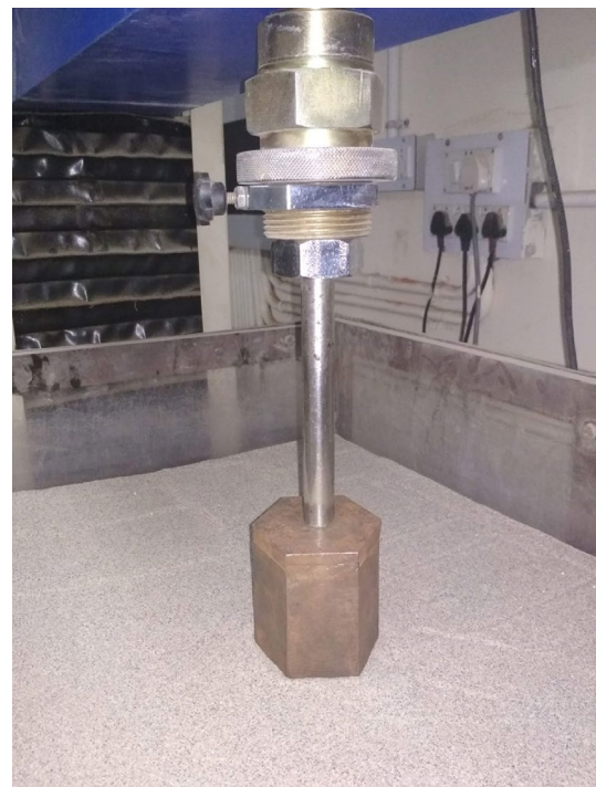
Fig. 5 Placement of skirted footing on sand bed
