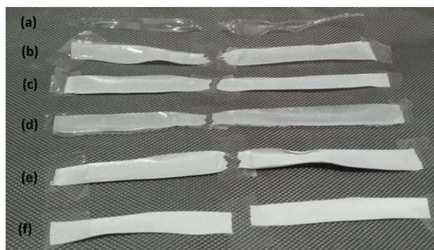
Fig. 8 Image of tested samples of PVA loaded with ZTA nanoparticles at a 0 wt%, b 0.5 wt%, c 1 wt%, d 1.5 wt%, e 2 wt% and f 2.5 wt%
