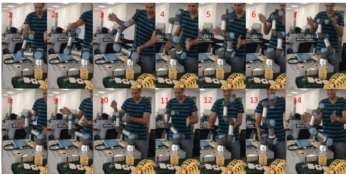
Fig. 3 Experiment demonstration under collision force
