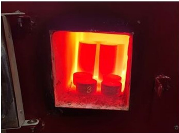
Fig. 2 Samples under furnace pre-treatment at 600 °C temperature
