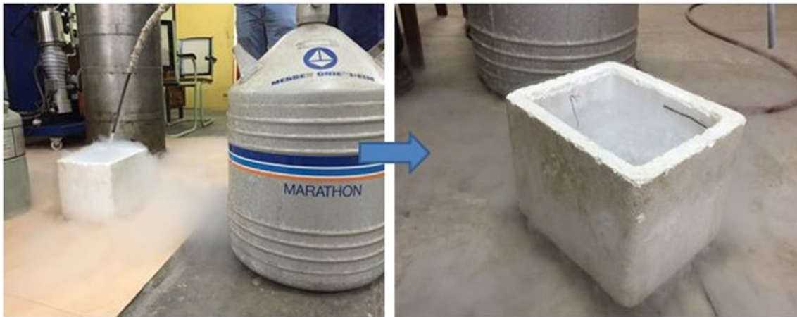
Fig. 3 Samples under cryogenic treatment using LIN
