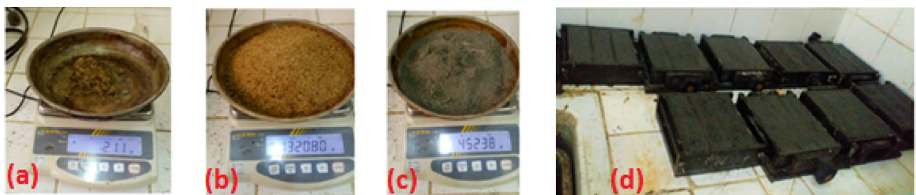
Fig. 3 Steps in the elaboration of fibro-cement mortar (FCM) samples (weighing and filling of moulds). Weighing of the different components of the sample d fiber cement mortar: a fiber, b sand, c cement
