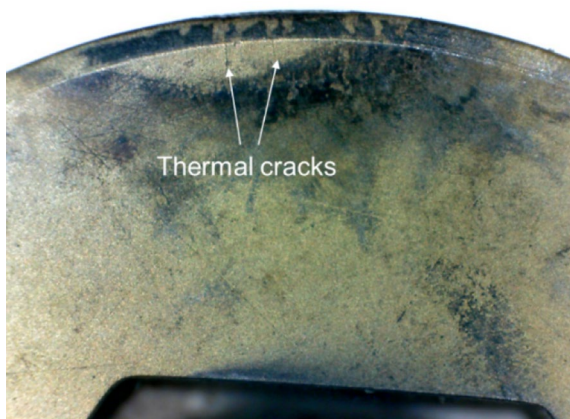
Fig. 17 Rake surface of insert 1 after 7 passes (expanded 80X)
