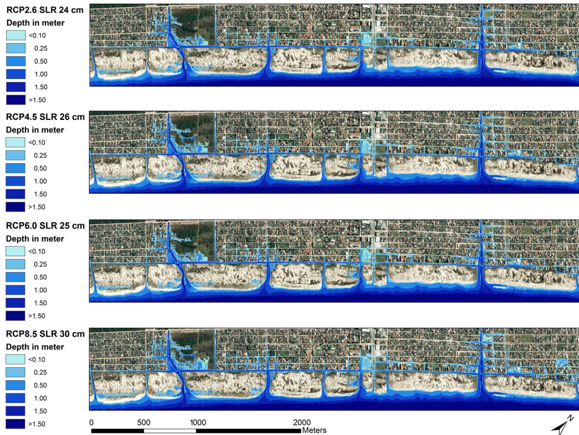
Fig. 9 Bathtub modeling for the 2046–2065 range of IPCC sea-level rise projections for Cassino Beach
