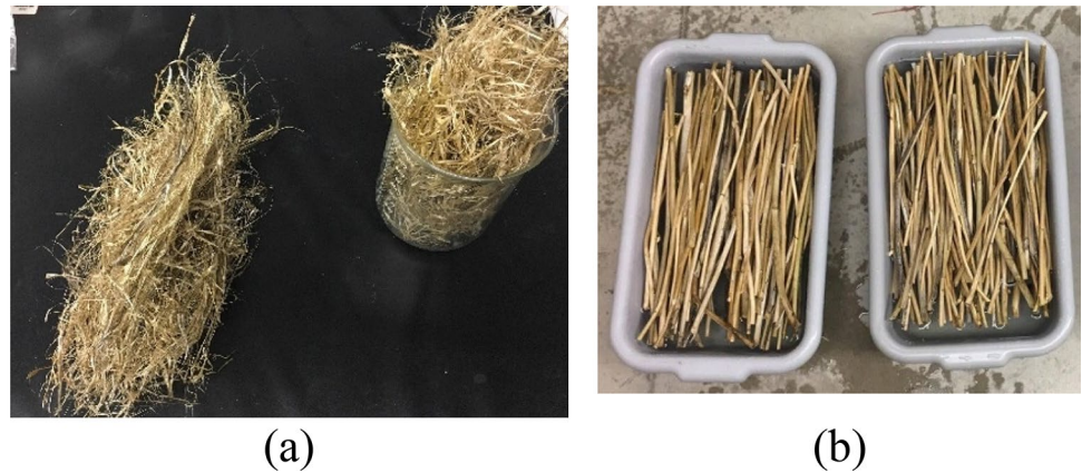
Fig. 3 Extracted raw canola fibres a from the water-retted plant stems b
