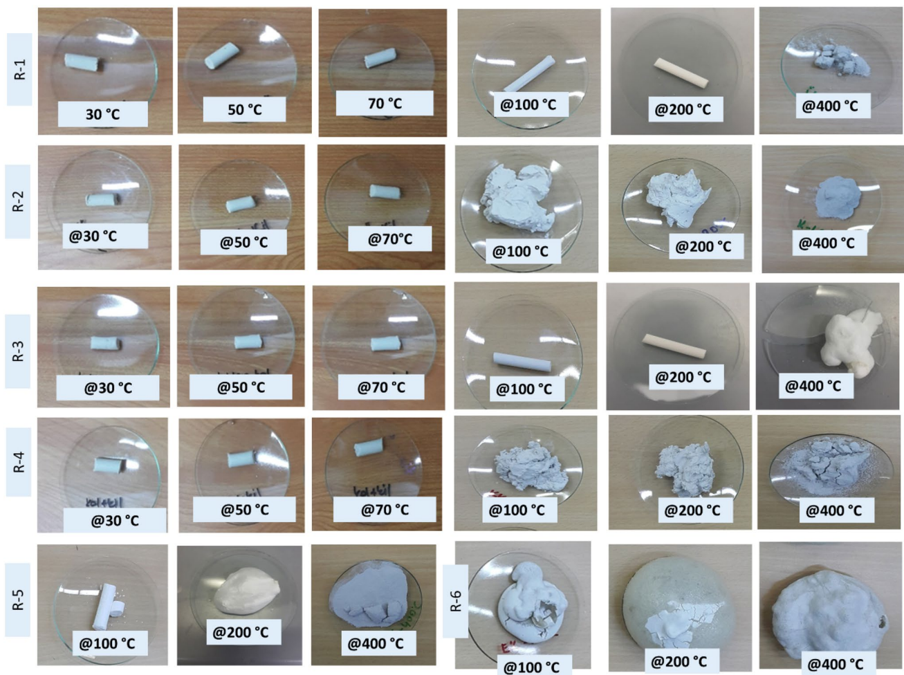
Fig. 1 Images of boron-based rods after thermal resistant test at low and high temperature
