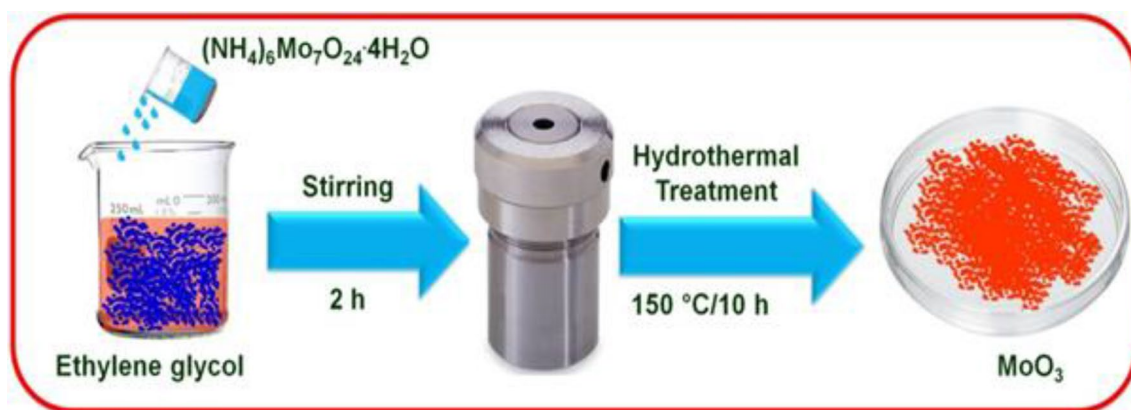
Scheme 1. Schematic representation of synthesis of \text{MoO}_3 nanorods
