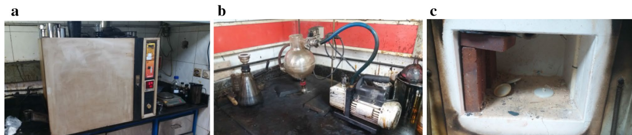
Fig. 3 Equipment used to measure the insolubility of CT in quinoline and toluene and coke value; oven modeling Binder (a), equipment of vacuum package included round-bottom flask and vacuum pump (b), electric heat furnace (c)
