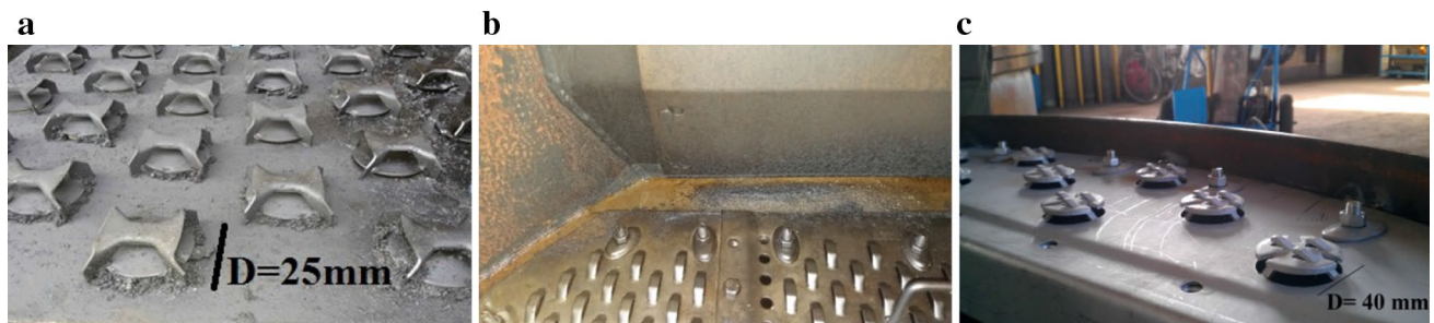
Fig. 6 Tray number 22 vacuum distillation column with 30 mm depth and 25 mm diameter movable valves (a, b), new design on tray number 22 by removing seal pan and inserting 40 mm diameter fixed valves (c)
