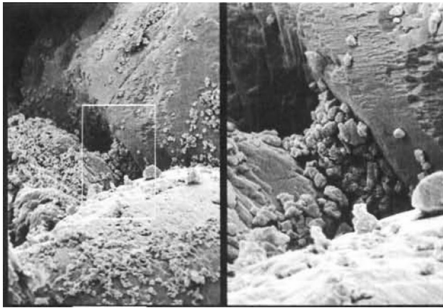
Fig. 2 Pore bridging and surface deposition reported by Todd et al. [5]
