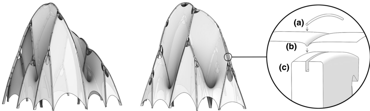
Fig. 14 Geometry of stretched fabric and detail of fabric attachment: a 3 mm nylon cord that presses b the fabric with sewn seam into c the timber arch with a continuous machined rebate
