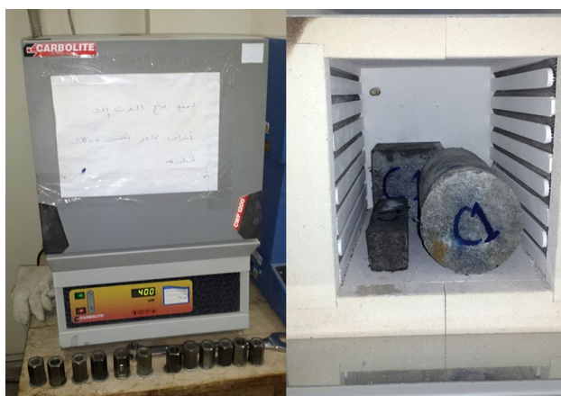
Plate 4 Furnace used in the heating regime
