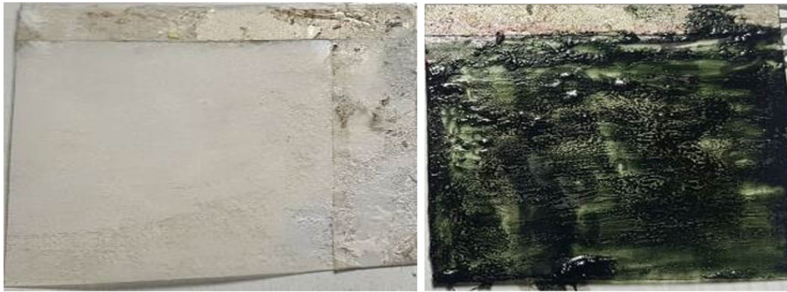
Fig. 2 ITO-PET substrate with the TiO 2 layer (left) and hydrogel with PANI during polymerization (right)
