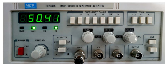
Fig. 12 Frequency measure using frequency counter
