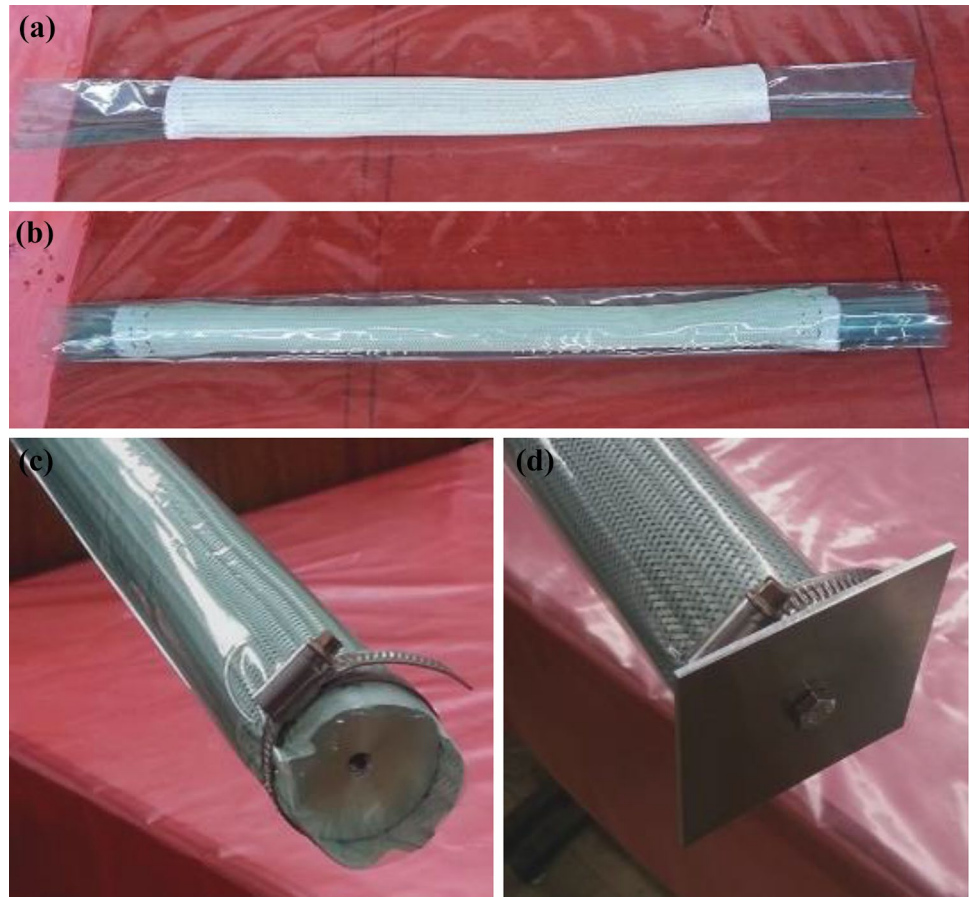
Fig. 1 Specimen preparation process. a Positioning of glass fiber sleeves on top of inner PE sleeve, b glass fiber sleeves enclosed between PE sleeves. c mounting of the lower metallic disc and clamp. d Installation of the bottom plate after O-ring placement
