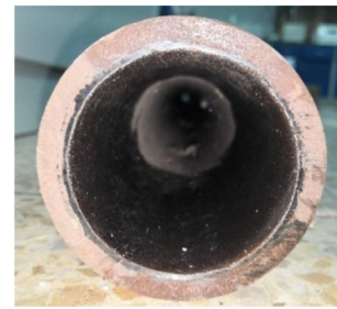
Fig. 6 A real product of ceramic-lined steel composite pipe
