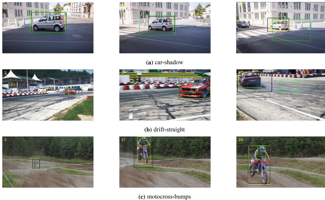
Fig. 3 Comparison between KCF and scale-variable KCF with APCE. The yellow rectangles represent groundtruth, the green rectangles represent the tracking results of the original KCF, and the black rec-
