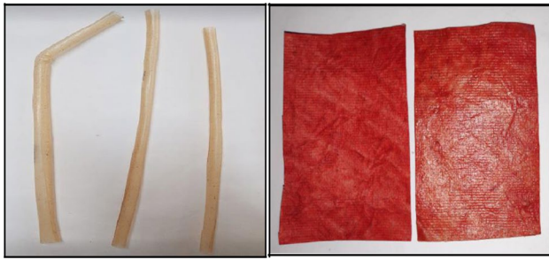
Fig. 7 Bioplastic straws and handmade paper without (left) and with bioplastic coating
