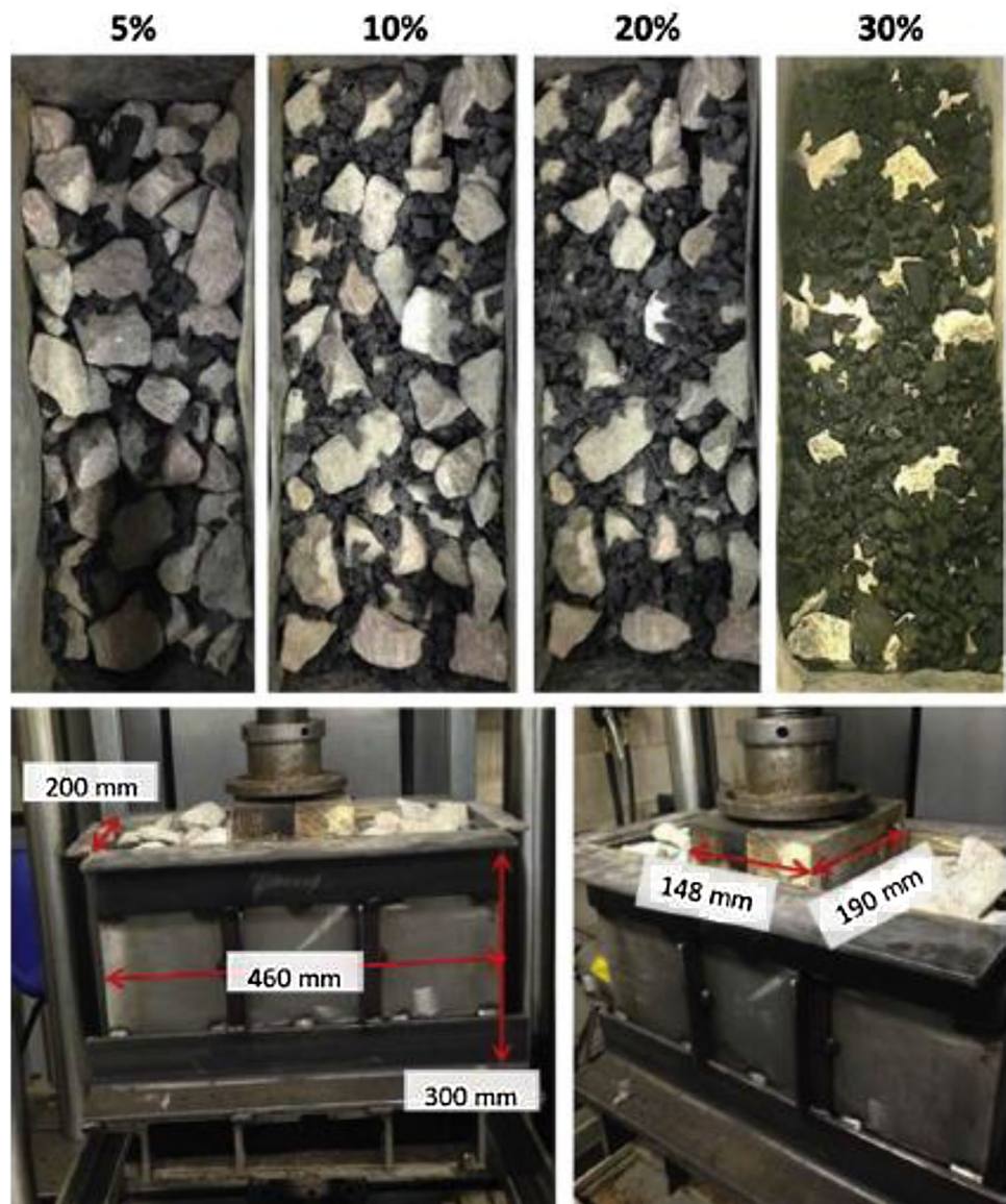
Fig. 20 Different percentages of rubber crumb mixed with ballast and large scale box test set up [107, 133]
