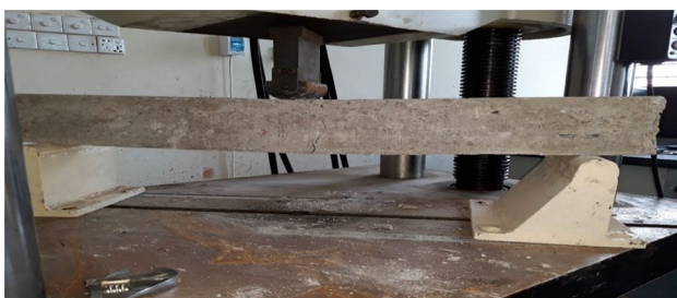
Fig. 3 Visible flexural cracks under point loading in RCBs
