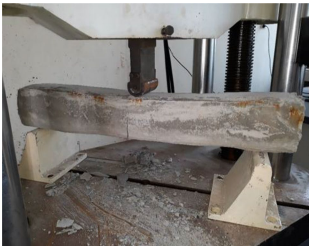
Fig. 7 Failure mode of W1-type beam
