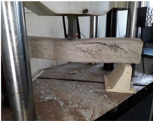
Fig. 9 Debonding failure in W2-type beam
