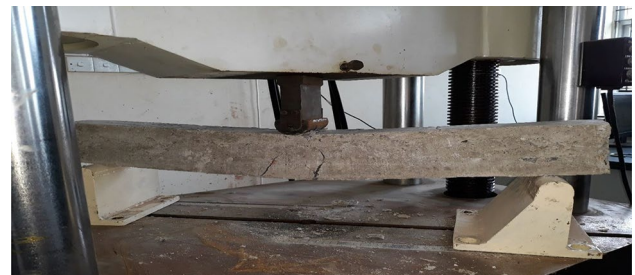
Fig. 4 Increased and widened flexural cracks with load in RCBs
