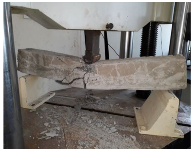
Fig. 8 Crack pattern in W3-type beam
