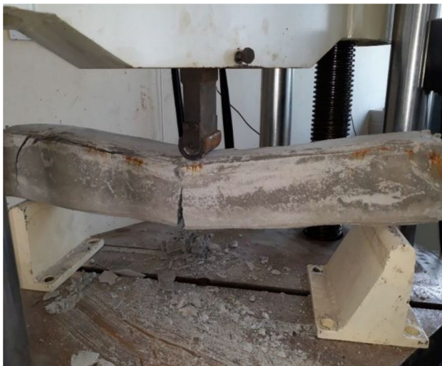
Fig. 10 Debonding and concrete crushing failure in W3-type beam
