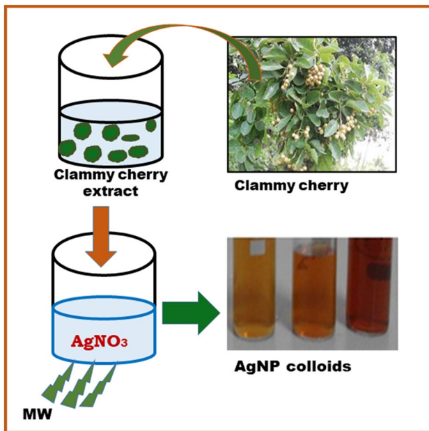
Fig. 1 Pictorial representation of MW assisted synthesis of AgNPs using clammy cherry extract
