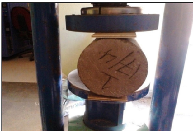
Fig. 5 Tensile strength test on cylinde
