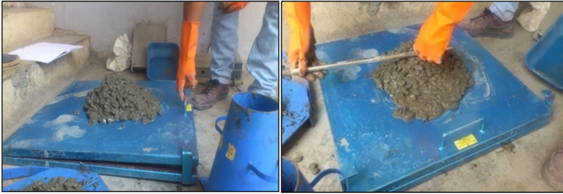
Fig. 3 Flow table test
