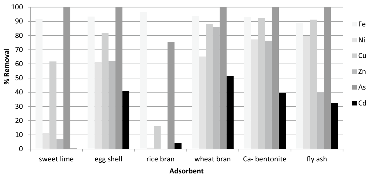
Fig. 1 Percentage removal of metal ions using different adsorbents
