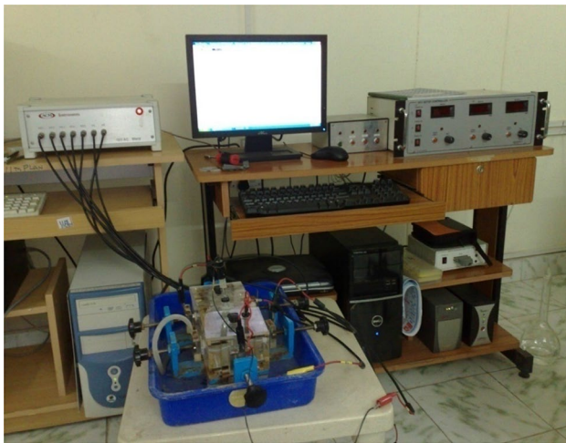
Fig. 2 Electrochemical system of GILL AC unit
