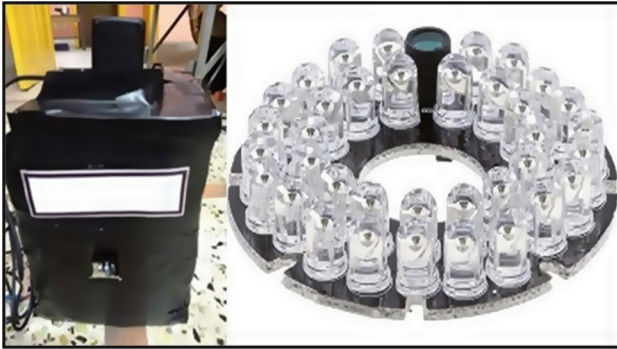
Fig. 7 Finger vein detector and NIR light
