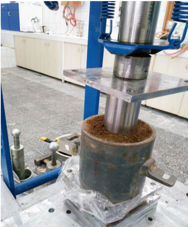
Fig. 3 Driving the sampler into the mold by hydraulic jack
