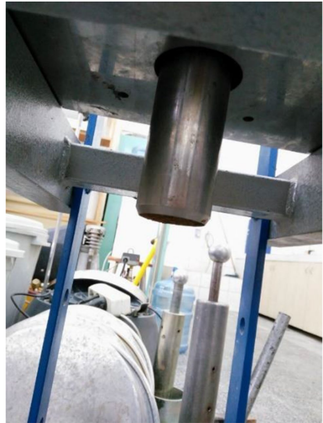
Fig. 4 Extracting down the specimen from the sampler with hydraulic jack
