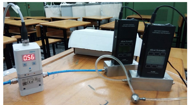
Fig. 5 Measuring with Alicat Scientific Brand M series mass flow meter
