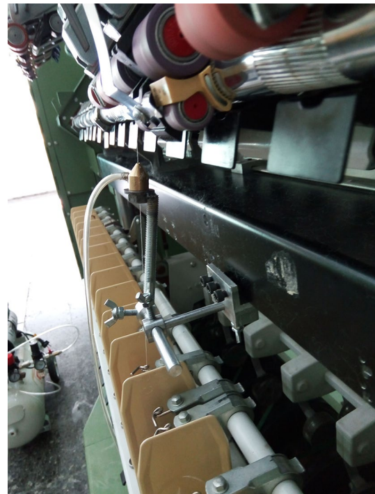
Fig. 1 Application of an air nozzle on the sirospun spinning system (siro-jet)
