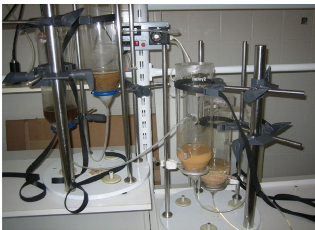
Fig. 2 Experimental laboratory model system for testing biocide treatment with the different resin beads
