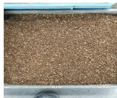
Fig. 3 Crushed coconut shell aggregates
