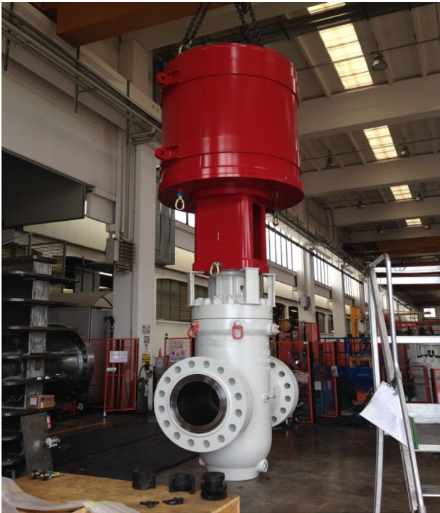
Fig. 5 Hydraulic actuator through conduit gate valve
