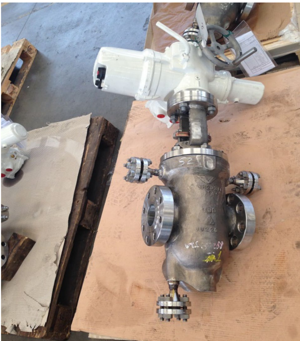
Fig. 6 Electrical actuated through conduit gate valve
