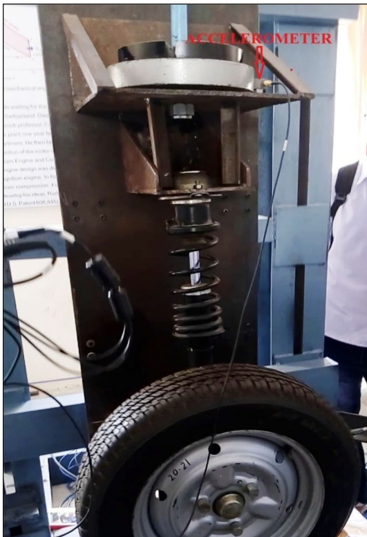
Fig. 3 Position of accelerometers—sprung mass
