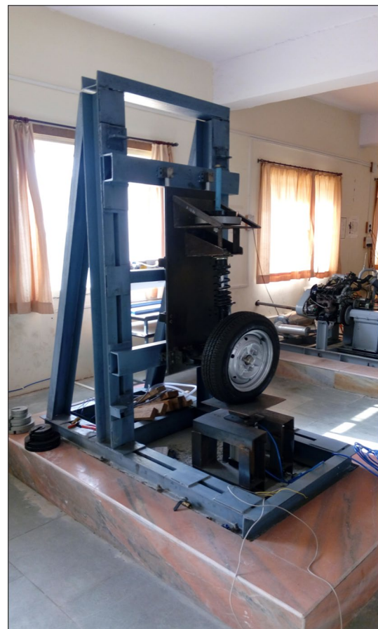
Fig. 2 Quarter car test rig
