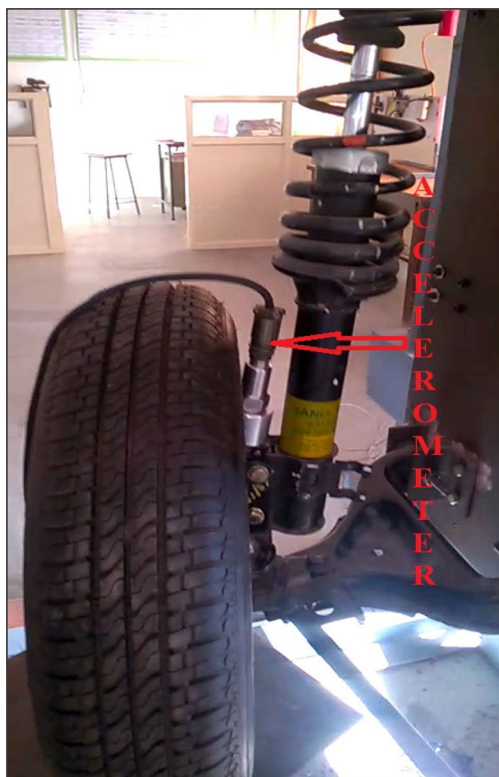
Fig. 4 Position of accelerometer—unsprung mass
