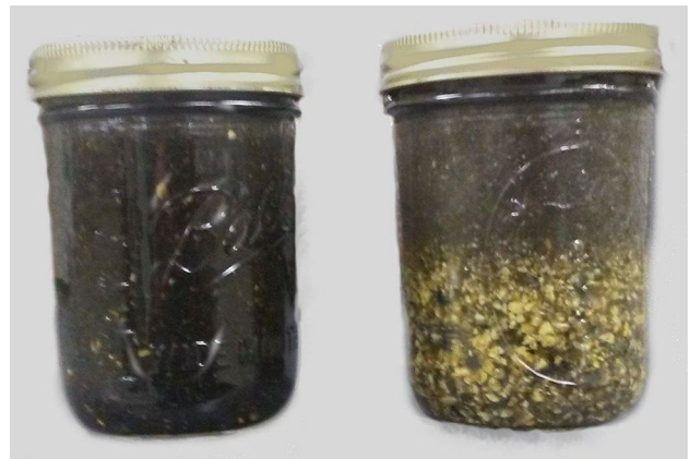
Fig. 3 Sludge samples removed from digesters at the end of trial three. Left, sludge removed from sound-treated digester, right, sludge sample removed from control digester
