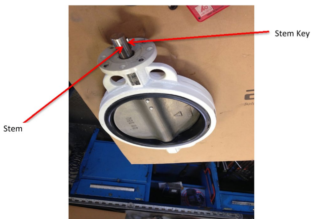
Fig. 2 Stem and stem key for a rubber-lined butterfly valve
