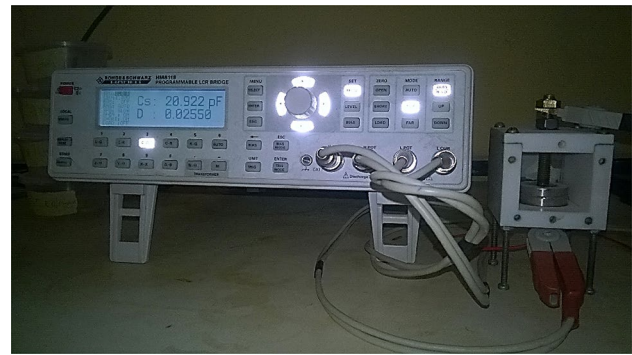
Fig. 2 Dielectric measurement test set-up
