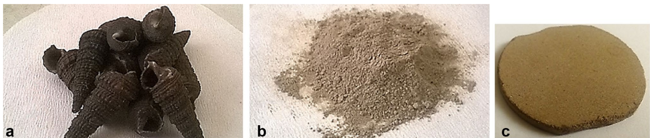
Fig. 1 Samples a periwinkle shell, b periwinkle shell powder and c periwinkle shell pellet
