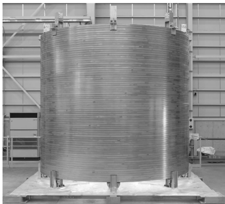
Fig. 17 Group photograph after fabrication of the final conductor
