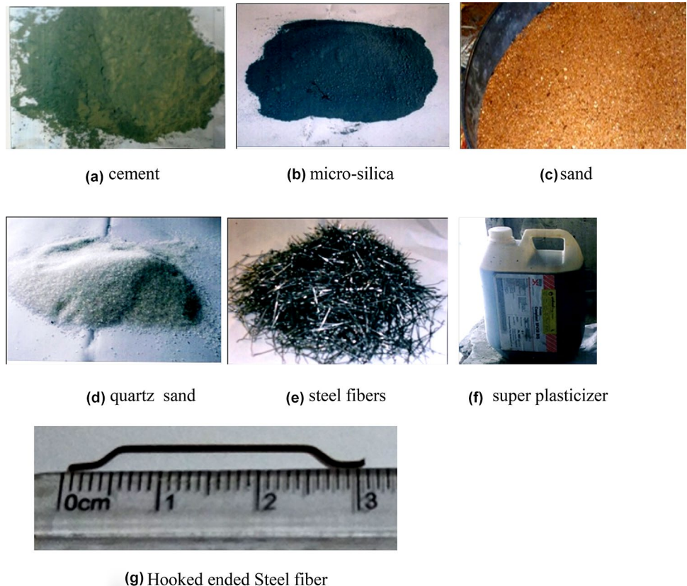
Fig. 1 Basic components of the fabricated UHPFRC
