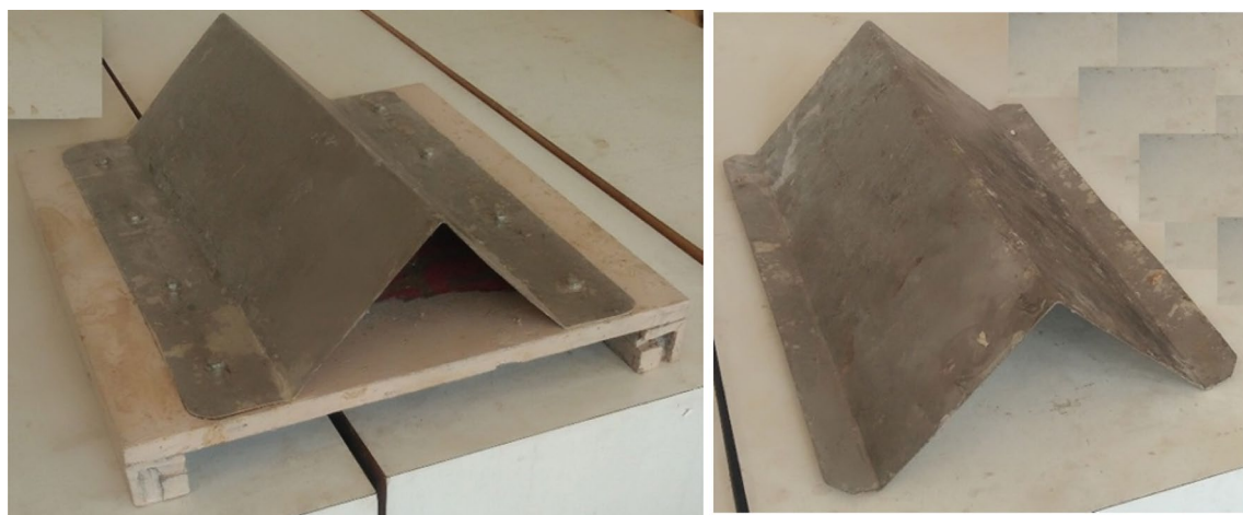
Fig. 2 Photographs showing bottom V-tool plate (left) and top V-tool plate (right)
