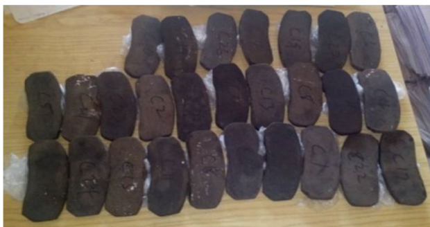
Fig. 2 Heat-treated coconut shell-reinforced brake pad samples
