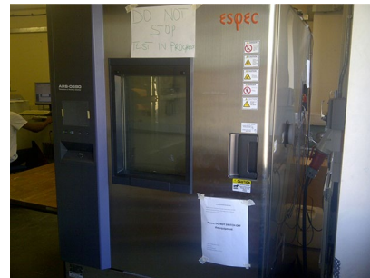
Fig. 5 ESPEC's ARS-0680 environmental chamber
