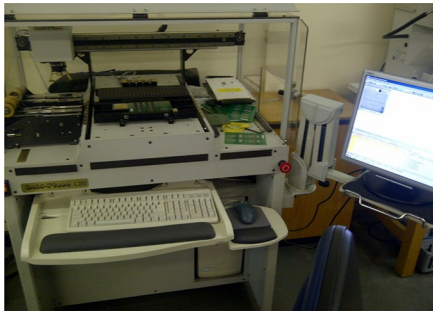
Fig. 2 Pick and place (PnP) machine for component placement
