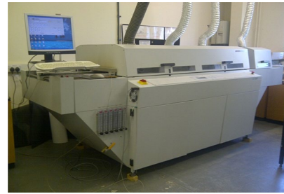
Fig. 4 Novastar 200HT convection reflow oven
