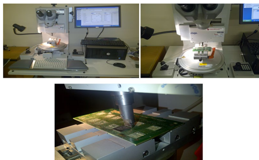
Fig. 6 Dage bond tester in operation during shear strength test
