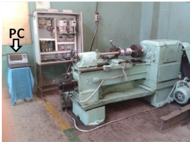
Fig. 12 Developed retrofitted CNC spinning machine
