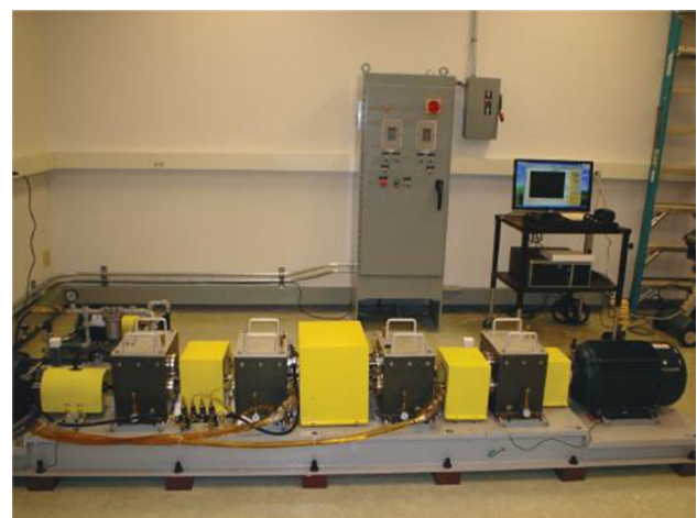
Fig. 6 Gear-train experimental setup
