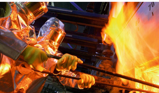
The production of specialty glasses is energy-intensive: they are melted at temperatures of up to 1,700 °C.
